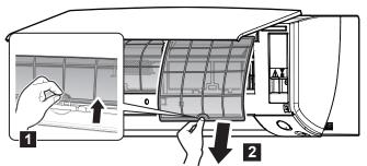
Remove the titanium apatite deodorising filter and the silver particle filter 3 from all 4 claws.
