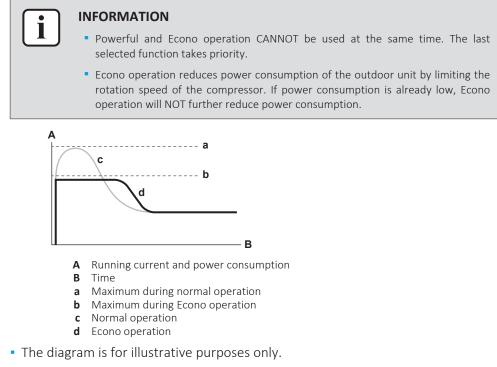
• The maximum running current and power consumption of the air conditioner in Econo operation varies with the connected outdoor unit.
